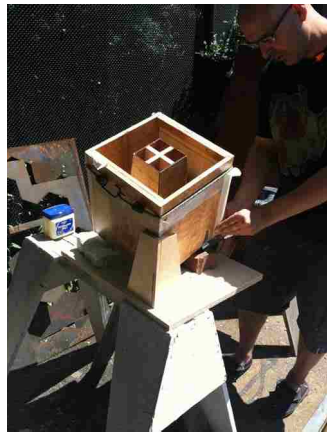
7. sealing edges using tape
